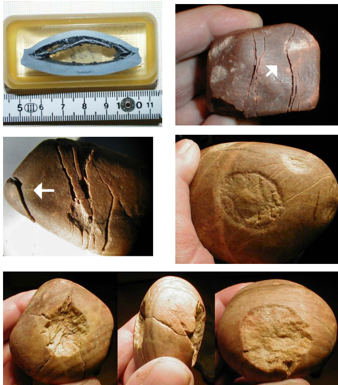
Fig.1. Spallation fractures in experimentally shocked ARMCO iron (a) and in naturally impact-shocked quartzite cobbles. b, c: Internal spall fractures and a nearly detached spall in c. d, e: Spallation craters. Note the central mound in d, and the opposite craters in e.
